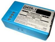
Electronic lapscoring is now the norm at most tracks for all classes excluding bikes, and it is likely you will need to purchase an Electronic Lapscoring Transmitter.
